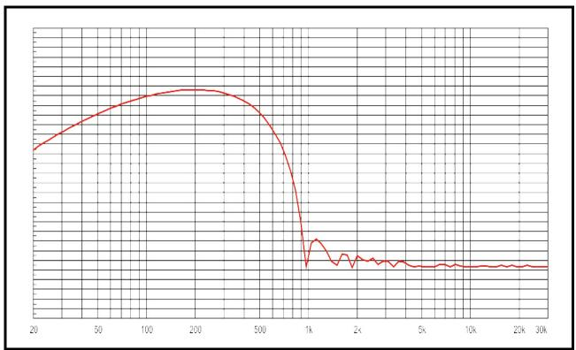
FIGURE 26. Frequency Response - Preset 1 (20Hz to 300Hz)
